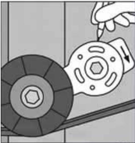
FIGURE 11: TENSIONER MARKING
